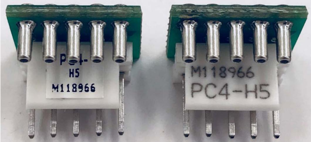
Side-by-side comparison of the current PC4-H5 labeling (left) and the new PC4-H5 laser marking (right).
