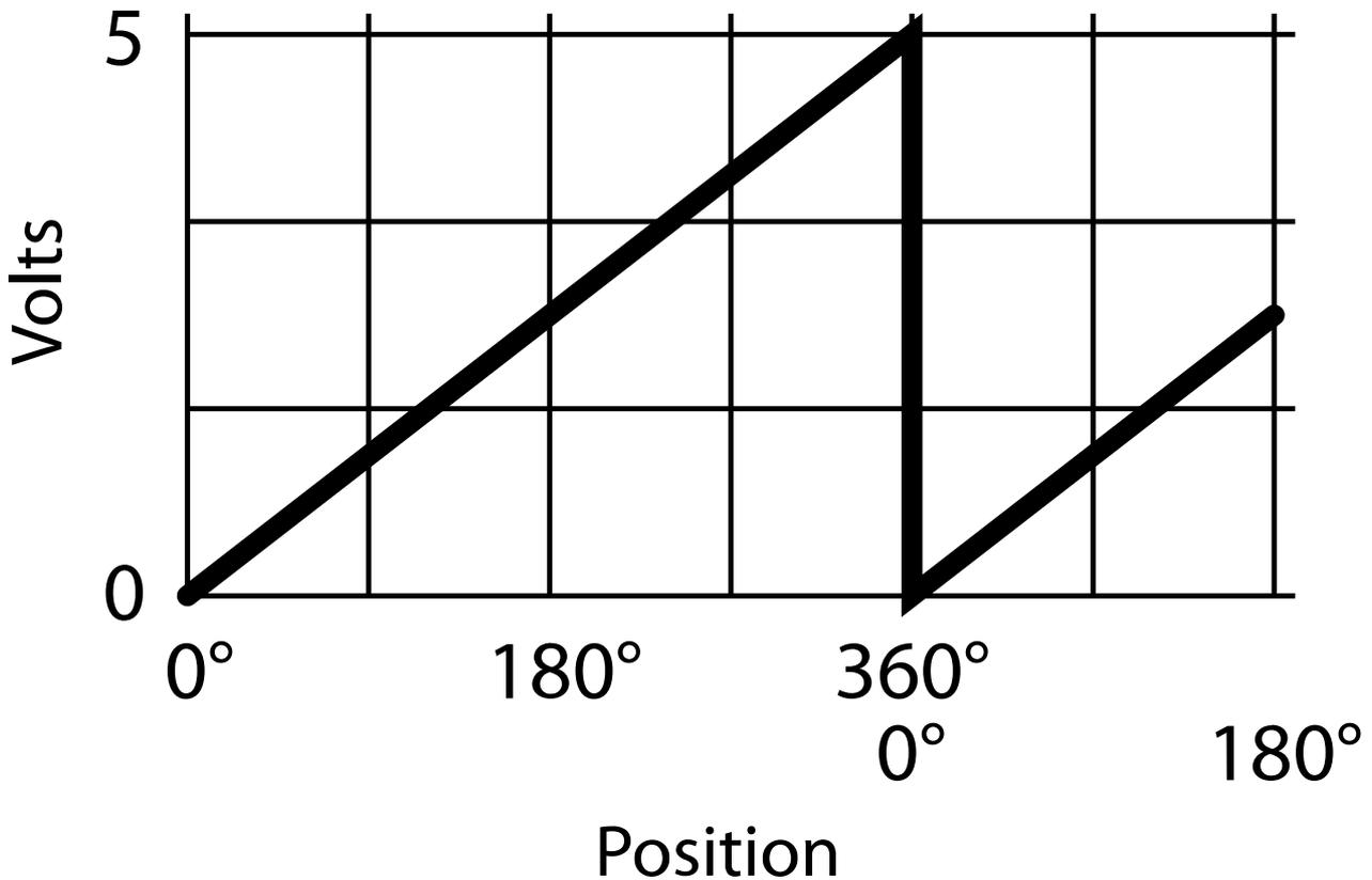
Analog output is only available in 10-bit resolution. The analog output voltage is ratiometric to the power supply voltage and will typically swing within 15 millivolts of the power supply rails with no output load. This non-linearity near the rails increases with increasing output loads. For this reason, the output load impedance should be  $\geq 4.7k\Omega$  and less than 100pF. The graphs below show the typical output levels for various output loads when powered by a 5V supply.
