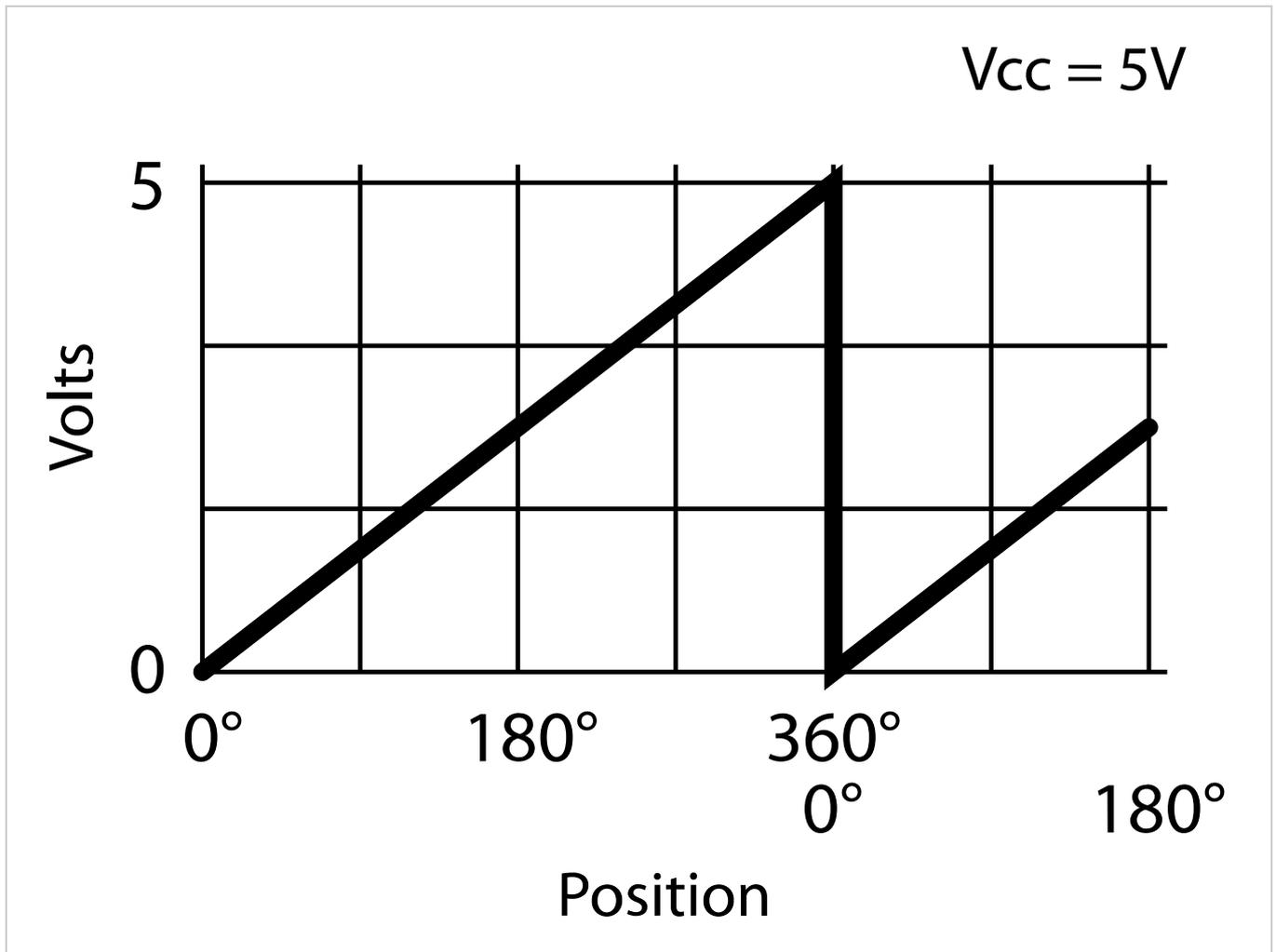
The analog output has 12-bit resolution. The analog output voltage is ratiometric to the power supply voltage, which is typically 5.0V
