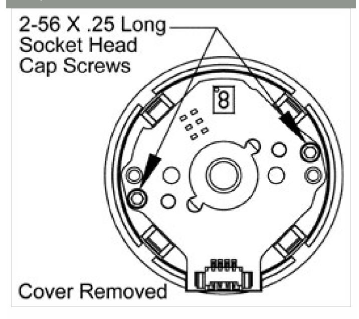
Provides two #2-56 x " screws in place of two #4-40 x 1/4".
