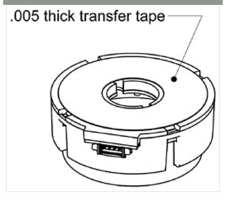
The **T**-option base provides a transfer adhesive (with peel-off backing) that may be used when mounting holes are not available. A centering tool is required when using this option.
