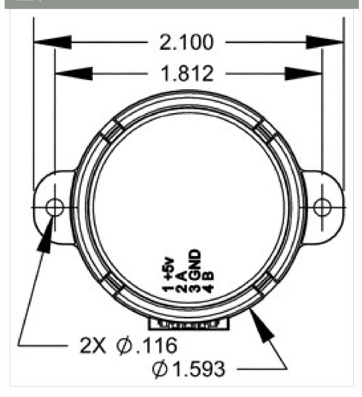
Provides mounting ears on the base allowing for a 1.812" bolt circle.
